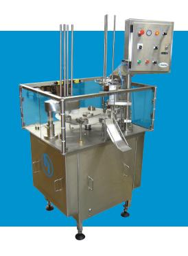
Fully automatic single track (intermittent motion rotary) filling and lidding system for liquids, pastes, creams, and other viscous products.
