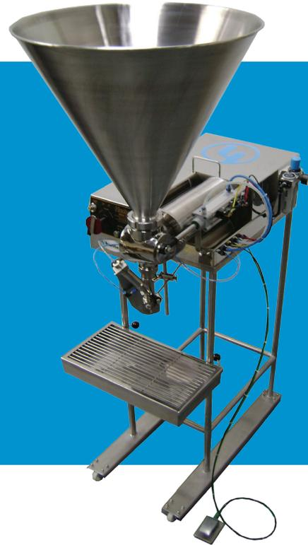
**Pneumatically operated piston filler for liquids, pastes, creams, and other viscous products.**
